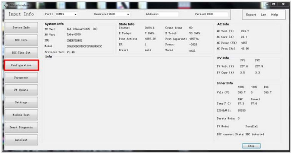
Figure.6. Indication of read information of inverter on ShineBus
